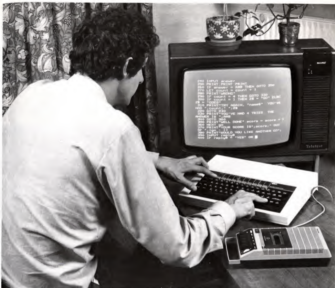
The BBC microcomputer in its simplest form, using a domestic television set as a display and an ordinary cassette tape recorder to record programs and to play them back.
